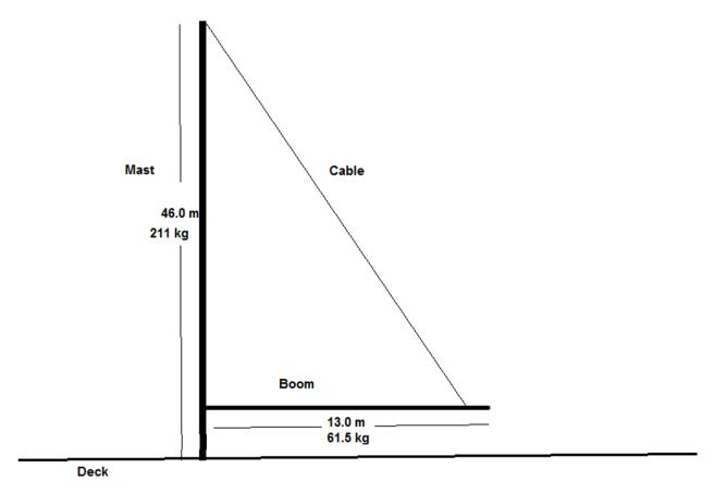
a) Draw a free body diagram of the boom in the space below, showing all forces acting on it.
